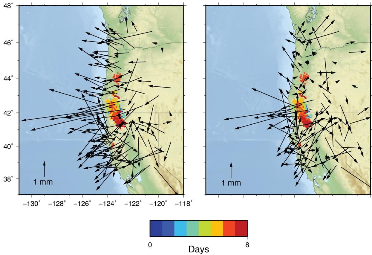
**Figure S1.** Map of displacements for ETS Event 9 (November 2018) before (left) and after (right) the removal of the common mode signal.
