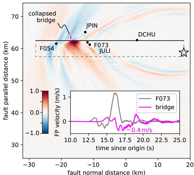
**Figure 6** Snapshot of modelled fault parallel ground velocity at 17.5 seconds. Inset shows the the velocity time history at F073 (grey) and the location of the collapsed Gaoliao bridge (magenta). The model shows large asymmetry in fault-parallel ground velocity across the fault. Lower amplitudes are predicted for the footwall side of the fault where the collapsed Gaoliao bridge is located (magenta) compared to F073 on the other side of the fault.
