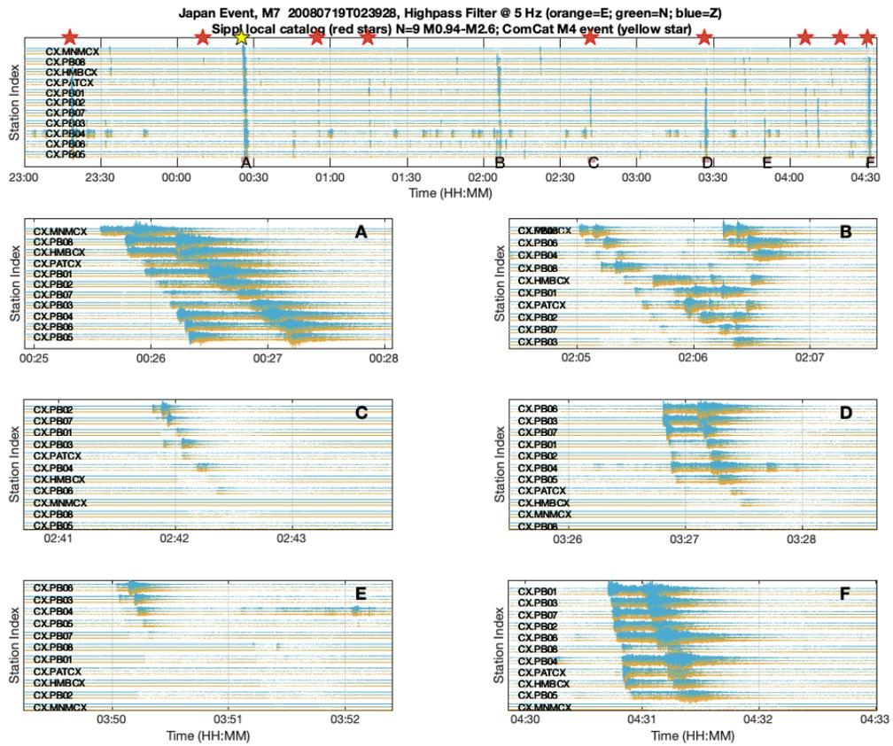
*Figure A. Example of the reformatting of the original Figure 6 (now Figure 7), where we now order the traces by the arrival times. In doing so, the move-out becomes more apparent.*
