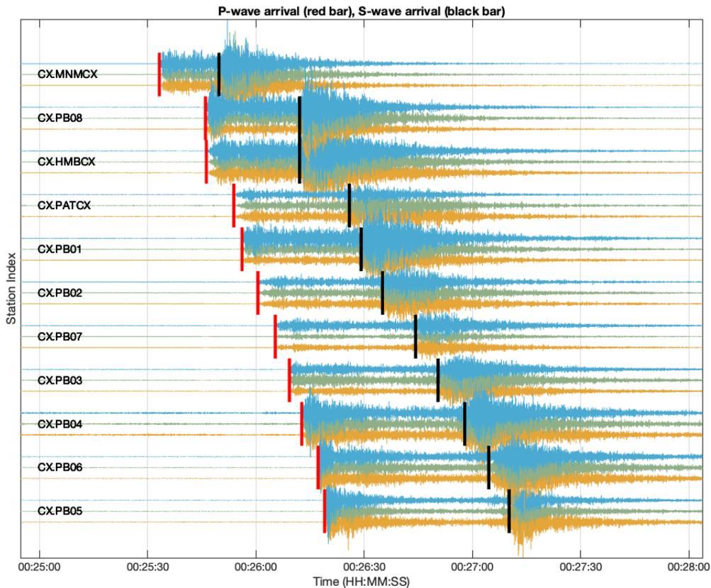
*Figure C. Data from the M4 2008-07-19 earthquake (part of Figure 7A). To determine seismic wave speeds, we identified P-wave (red bars) and S-wave (black bars) arrival times. Figure for illustrative purposes only to respond to the reviewer’s question. This figure is not included in the updated manuscript.*
