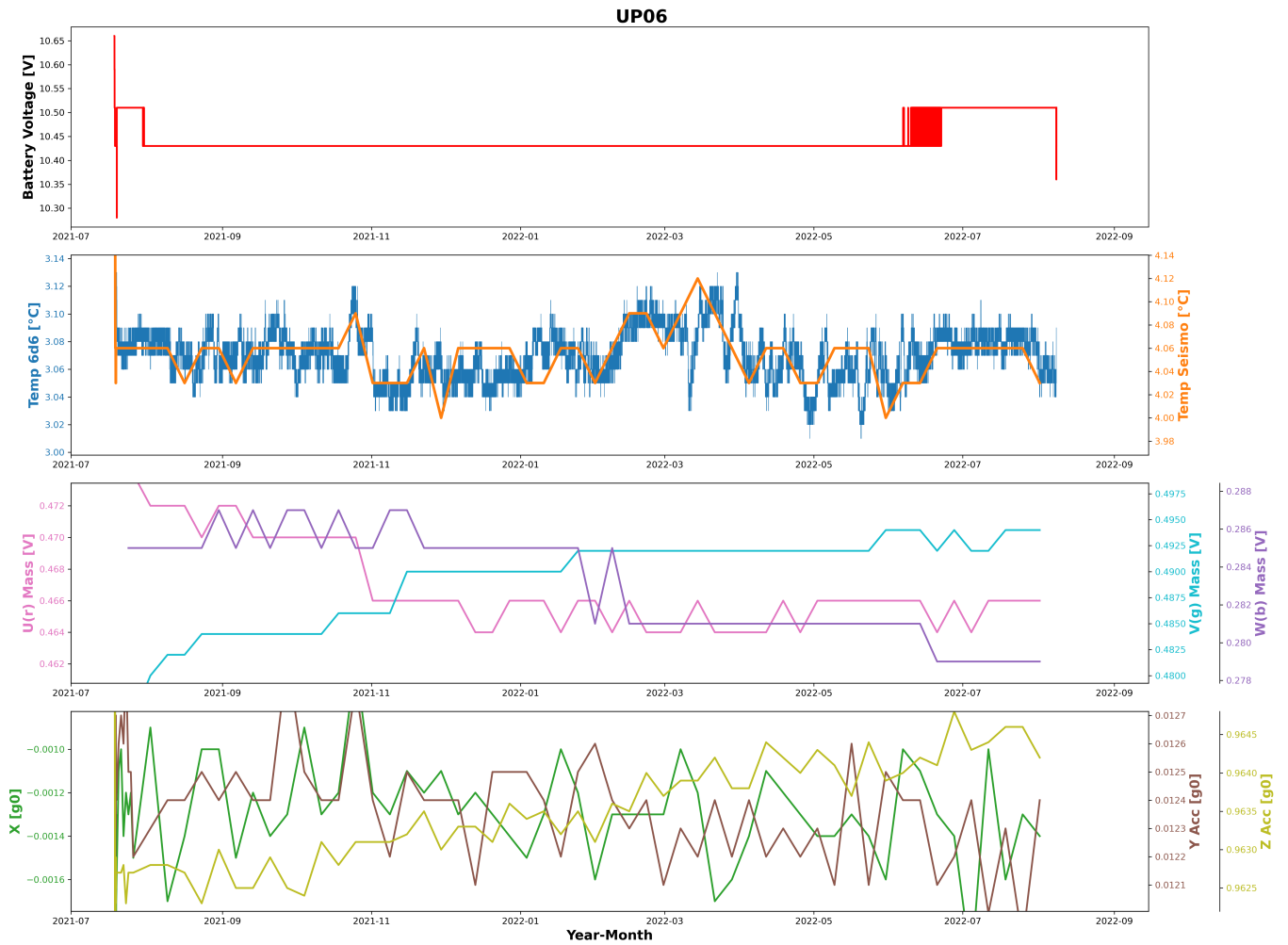
Figure S 2 Illustrative example of state-of-health data for station UP06. The top panel shows battery voltage, the second panel shows temperatures measured from the 6d6 recorder and the seismometer, the third panel shows mass, and the lowest panel shows static sensor acceleration. Note the different scales for each coloured graph. Most variations are small (check the actual values on the y-axis), and in the case of the third and fourth panels, scales plotted between -1 and 1 would not show apparent changes. For more examples of SOH plots, please refer to the additional online materials .
