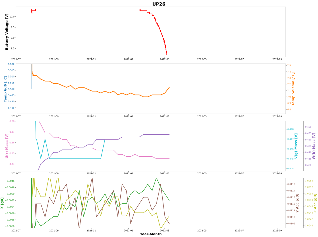
Figure S 5 Same as Fig. S2 but for station UP26. As explained in the main text, the temperature, mass position and static sensor acceleration show normal behaviour, but the battery was depleted earlier than expected, which suggests the insufficient capacity of the battery packs at the experiment's outset.
