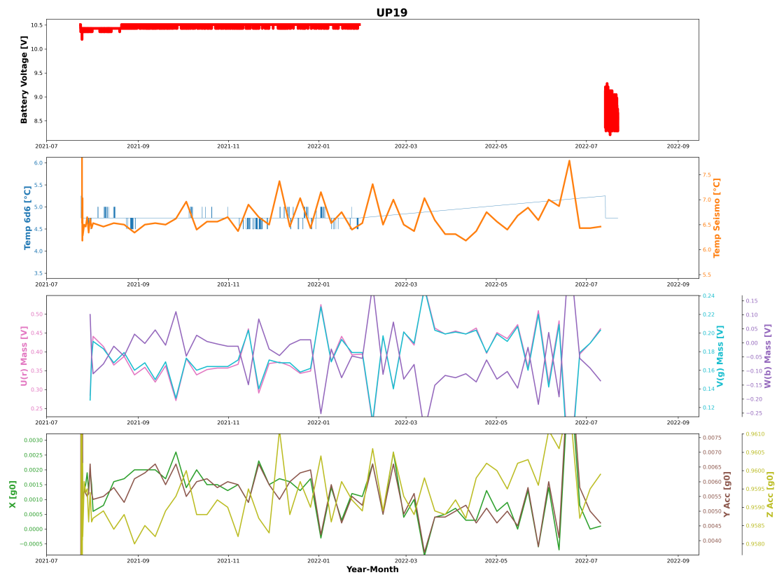
Figure S4 Same as in Fig. S2 but for station UP19. The mass voltage (2nd panel) and seismometer temperature (3rd panel) show significant variations, while the temperature of the data logger remained relatively constant. The OBS might have moved or tilted during deployment, leading to the battery being depleted earlier than expected (top panel). See the main text for further details.
