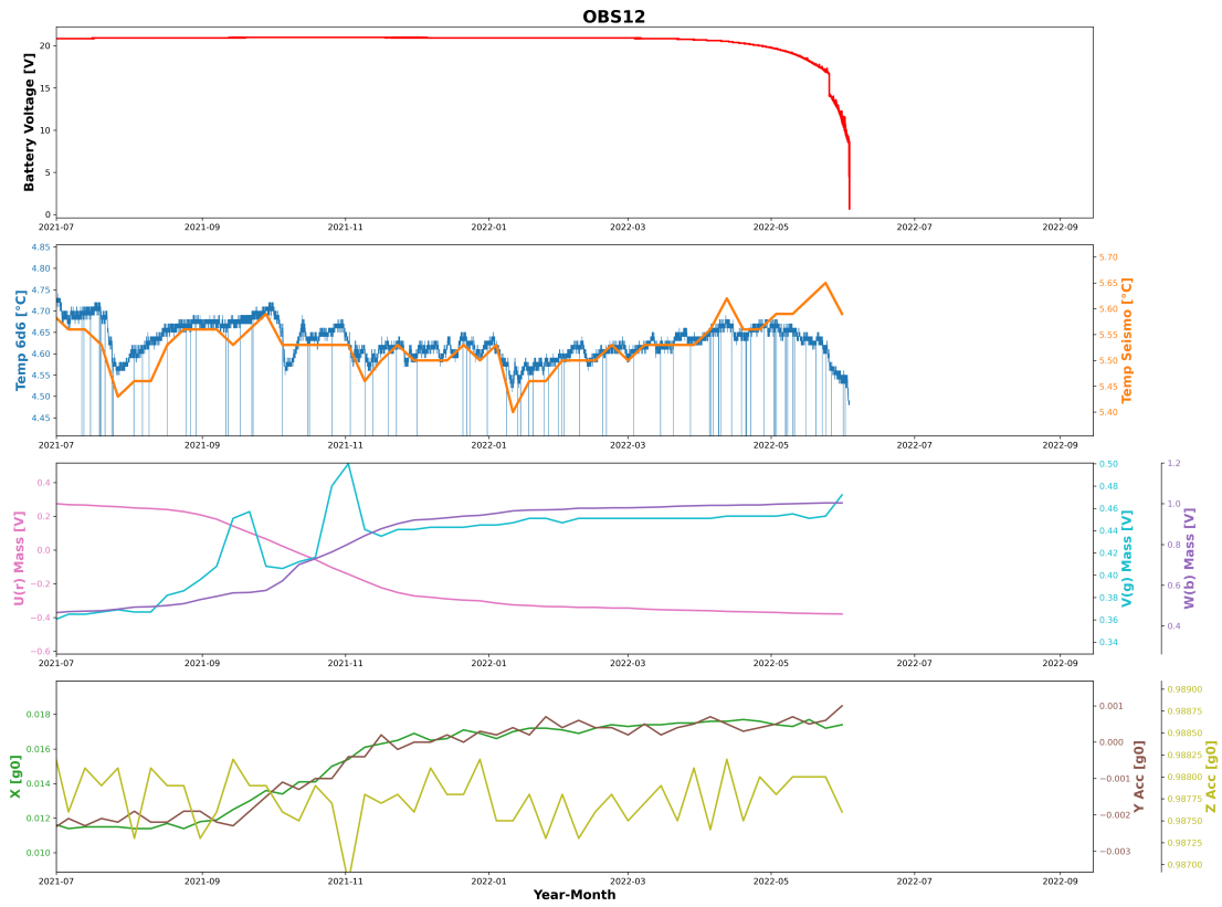
Figure S3 Same as in Fig. S2 but for station OBS12. In this case, the two bottom diagrams indicate the tilting of the instrument.
