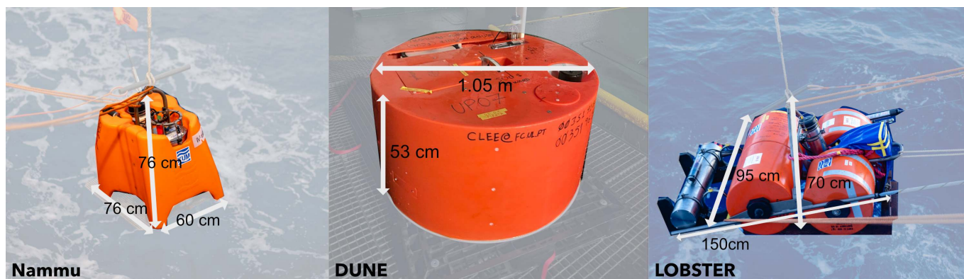
Figure 2 Comparison of OBS types used in the UPFLOW experiment. From left to right: NAMMU (provided by DEPAS and DIAS), DUNE (prototype provided by IDL), and LOBSTER (provided by DEPAS, GEOMAR, and ROA-UCM). Note that a new deployment configuration was used on all LOBSTER OBS (except for GEOMAR stations), where custom-made blue tarpaulin sheets secured the buoys towards the frame to minimise rope resonance.
