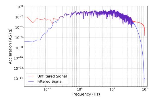
Figure. Comparison of the Fourier Amplitude Spectrum (FAS) for unfiltered (red) and filtered (blue) acceleration time histories. The unfiltered signal shows elevated low-frequency content due to noise and baseline trends.
