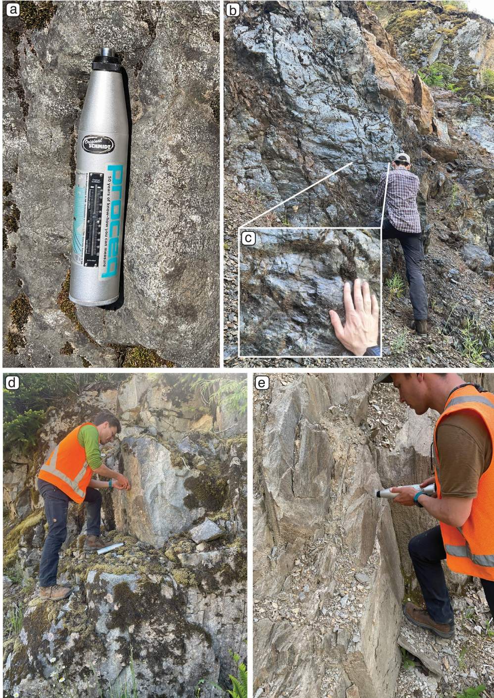
Figure S19: Photographs from the Schmidt hammer data collection. a) Proceq N-type Schmidt hammer used for data collection. b) Sub-vertical fault shear zone located near the uphill facing scarp. c) Close-up of the serpentinized material. Some near-horizontal slickenlines present. d) Cleaning the surface for Schmidt hammer sampling. e) Taking a sample, most samples were collected from near vertical surfaces along roadsides.
