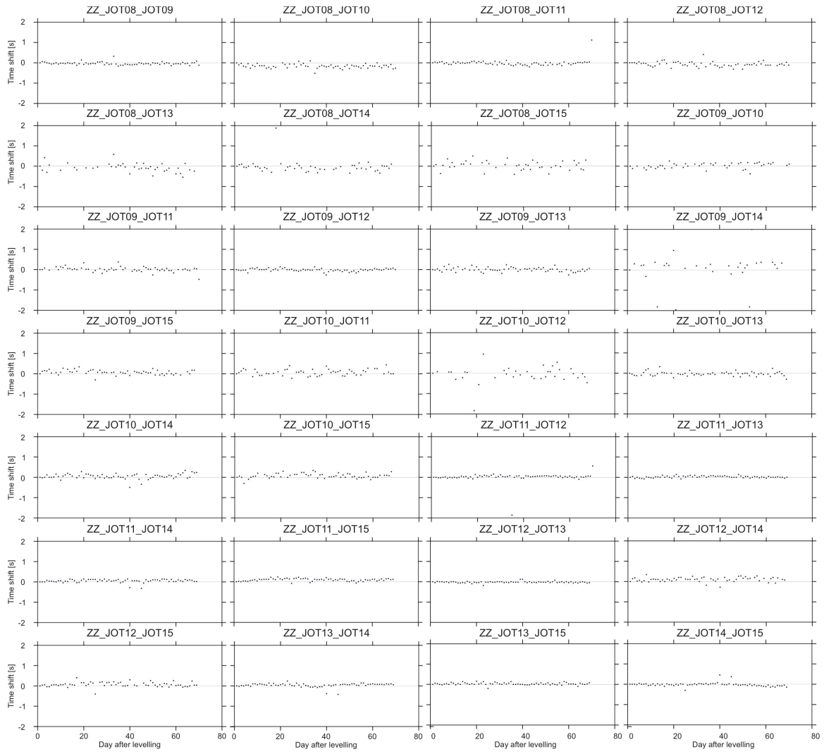
Figure S6. Time shifts derived from noise cross-correlations between short-term station pairs after clock drift correction. Caption see Fig. S4.
